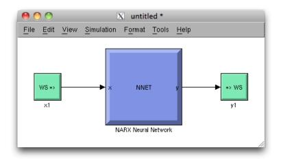
Simulink neural network blocks now allow initial conditions for input and layer delays to be set directly by double-clicking the neural network block. setsiminit and getsiminit provide command-line control for setting and getting input and layer delays for a neural network Simulink block.
