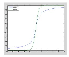
To set up a neural network to use the elliotsig transfer function, change each tansig layer's transfer function with its transferFcn property. For instance, here a network using elliotsig is created, viewed, trained, and simulated:
